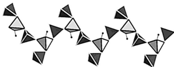
**Figure 7.** Open-branched vierer-single chain  $\frac{1}{4}[\text{BP}_2\text{O}_8(\text{OH})]^{4-}$  in the crystal structure of **2** ( $\text{BO}_4$  tetrahedra, gray;  $\text{PO}_4$  tetrahedra, dark gray; H, small pale gray spheres).
