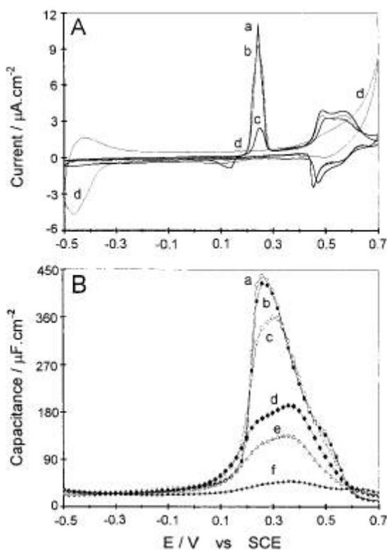
Fig. 5. Cyclic voltammograms (A) and capacitance versus potential curves (B) of Au(111) in 50 mM  $\text{NH}_4\text{Ac}$  (pH=4.6) containing cysteine (a) 0, (b)  $1.0 \times 10^{-7}$ , (c)  $5 \times 10^{-7}$ , (d)  $1.0 \times 10^{-6}$ , (e)  $2.0 \times 10^{-6}$ , (f)  $5 \times 10^{-6}$  M. Scan rate  $50 \text{ mV} \cdot \text{s}^{-1}$  for the CVs.
