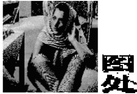
(3) Digital watermark image after compression and Extracted digital watermark after compression
