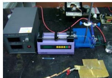
Figure 2. Electrospinning process and related machines
