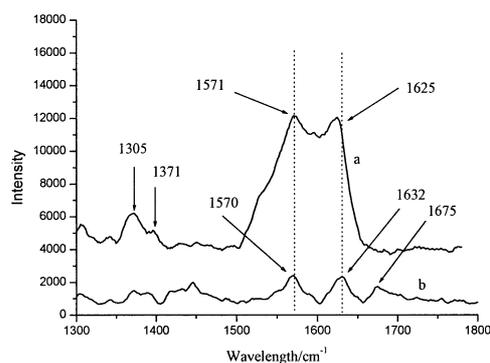
Fig. 5 RRS spectra of SiO<sub>2</sub>-hemin composite nanoparticles. a, SiO<sub>2</sub>-hemin composite nanoparticles; b, free hemin.
