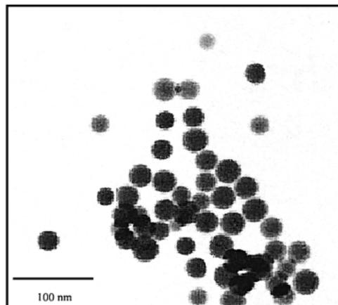
Fig. 3 TEM image of  $\text{SiO}_2$ -hemin composite nanoparticles.
