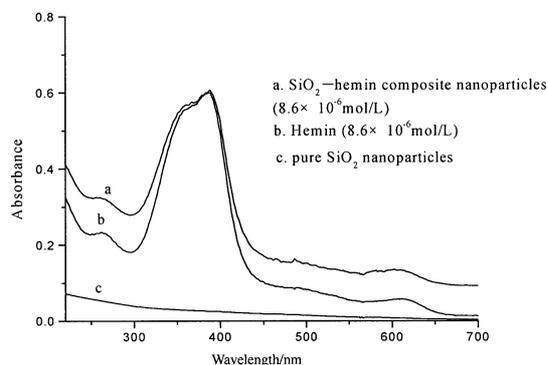
Fig. 4 UV-Vis spectra of SiO<sub>2</sub>-hemin composite nanoparticles.
