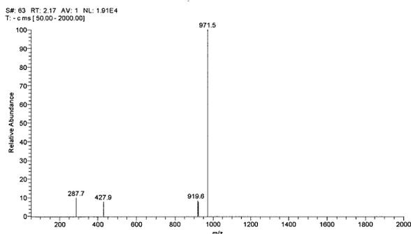
Fig. 2 MS spectrum of hemin functionalized precursor.
