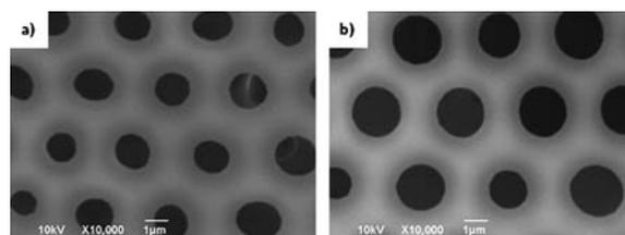
**Fig. 3** SEM images of PM<sub>2k</sub>-*b*-PS<sub>8k</sub> honeycomb films fabricated in different relative humidities. (a) 70% RH; (b) 80% RH.
