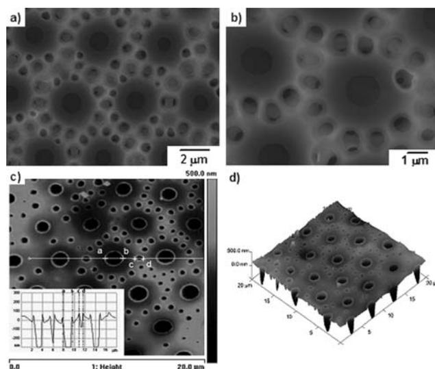
**Fig. 6** SEM and AFM images of  $\text{PM}_{2k}\text{-}b\text{-PS}_{10k}$  film fabricated at 28 °C in 50% RH (a) SEM top view of film; (b) magnified image of (a); (c) AFM height image (inset: section analysis of the white straight line); (d) 3D AFM image of film.
