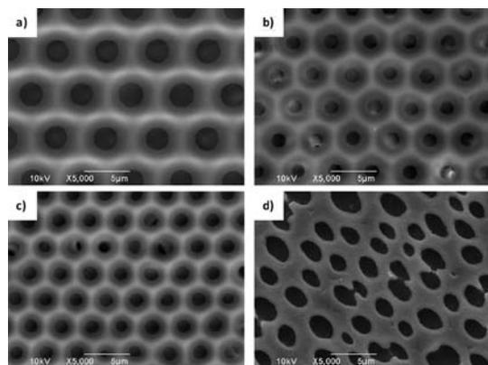
**Fig. 1** SEM images of porous PM-*b*-PS films fabricated *via* the casting/BF method at 20 °C in 50% RH. (a) PM<sub>2k</sub>-*b*-PS<sub>10k</sub>; (b) PM<sub>2k</sub>-*b*-PS<sub>8k</sub>; (c) PM<sub>2k</sub>-*b*-PS<sub>5k</sub>; (d) PM<sub>2k</sub>-*b*-PS<sub>2k</sub>.
