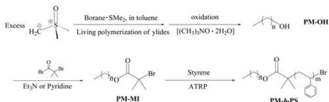
**Scheme 1** Synthesis of polymethylene-*b*-polystyrene (PM-*b*-PS) via a combination of living ylides polymerization and ATRP of styrene.<sup>18</sup>
