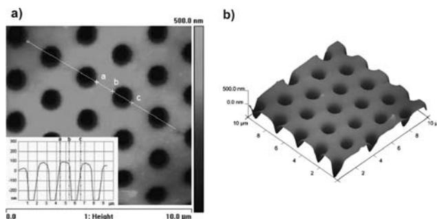
**Fig. 2** AFM images of PM<sub>2k</sub>-*b*-PS<sub>5k</sub> honeycomb film. (a) height image (inset: section analysis of the white straight line); (b) 3D image of film.
