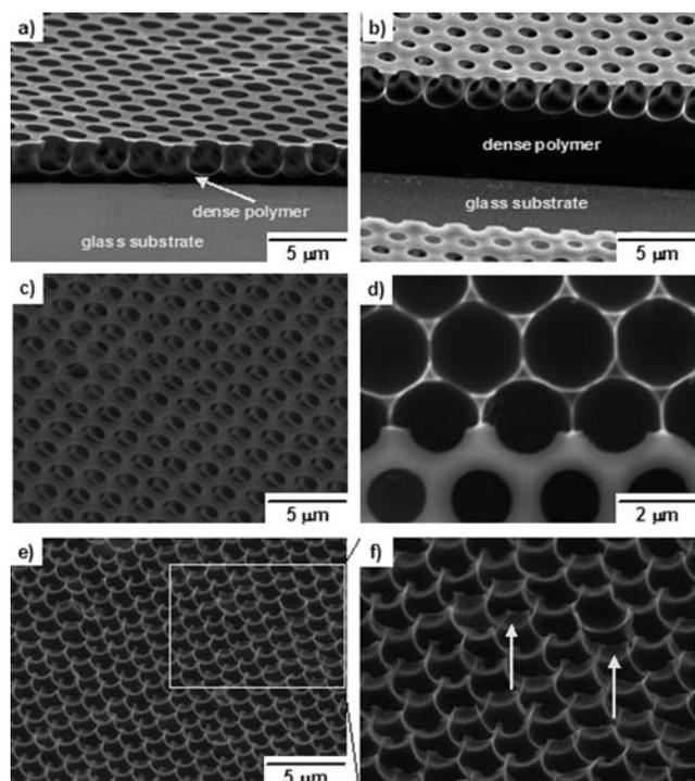
**Fig. 4** SEM images of honeycomb films of  $\text{PM}_{2k}\text{-}b\text{-PS}_{10k}$ . (a) and (c)–(f)  $\text{PM}_{2k}\text{-}b\text{-PS}_{10k}$  film fabricated by the dipping/BF method at 20 °C in 50% RH; (b)  $\text{PM}_{2k}\text{-}b\text{-PS}_{10k}$  film fabricated by the casting/BF method at 20 °C in 50% RH; (c) side view at tilt angle 40°; (d) top view; (e) pincushion structure (side view at tilt angle 40°); (f) magnified local view of (e).
