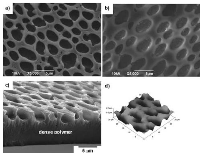
**Fig. 5** SEM and AFM images of  $\text{PM}_{2k}\text{-}b\text{-PS}_{2k}$  film. (a) and (b) top view; (c) side view; (d) 3D AFM image.
