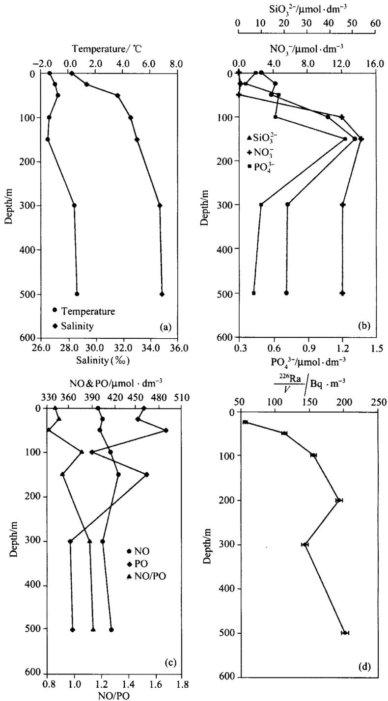
Fig. 6. The vertical profiles of  $^{226}\text{Ra}$  and other parameters at Station C39. (a) Temperature ( $^{\circ}\text{C}$ ) and salinity ( $\text{‰}$ ); (b) nitrate phosphate and silicate ( $\mu\text{mol}/\text{m}^3$ ); (c) NO, PO ( $\mu\text{mol}/\text{m}^3$ ) and NO/PO; (d)  $^{226}\text{Ra}$  specific activity ( $\text{Bq}/\text{m}^3$ ). Designators are the same as in fig. 5.
