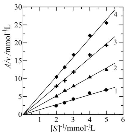
Fig. 8 Plot of  $A/v$  versus  $1/[S]$ . The final formaldehyde concentration for curves 1-4 are 0.5, 1.0, 1.5 and 2.0 mol·L<sup>-1</sup>, respectively.
