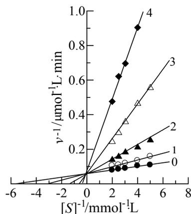
**Fig. 4** Lineweaver-Burk plots for the hydrolysis of pNP- $\beta$ -D-GlcNAc by the enzyme in different concentrations of formaldehyde. The formaldehyde concentration for lines 0-4 was 0, 0.5, 1.0, 1.5 and 2.0 mol · L<sup>-1</sup>, respectively. The assay conditions were the same as Fig.1.
