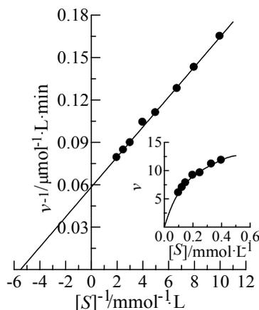
**Fig. 1** Lineweaver-Burk plot for the determination of  $K_m$  and  $V_m$  for NAGase on the hydrolysis of pNP- $\beta$ -D-GlcNAc. Conditions were 2 mL system containing  $0.1 \text{ mol} \cdot \text{L}^{-1}$  sodium phosphate buffer (pH6.2) at  $37^\circ\text{C}$ . The enzyme final concentration was  $0.01 \mu\text{mol} \cdot \text{L}^{-1}$ . The inset showed the relationship between the initial rate and the substrate concentration.
