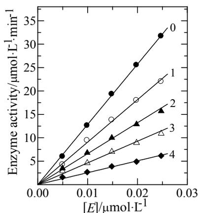
**Fig. 3** Effects of the enzyme concentration on its activity at different concentrations of formaldehyde. The concentrations of formaldehyde for curves 0-4 were 0, 0.5, 1.0, 1.5 and 2.0 mol·L<sup>-1</sup>, respectively. Assay conditions were the same as in Fig.2.
