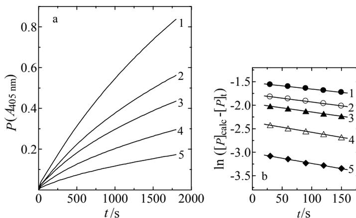
**Fig. 6** Determination of the inactivation rate constants for enzyme inactivation in 1.0 mol·L<sup>-1</sup> of formaldehyde solution. (a) Substrate reaction courses of the enzyme. Curves 1-5 are progress curves with 0.50, 0.40, 0.33, 0.25 and 0.20 mmol·L<sup>-1</sup> of substrate, respectively. The assay conditions were the same as Fig. 1. (b) Semilogarithmic plot of  $\ln([P]_{\text{calc}} - [P]_t)$  against time. Data were taken from curves 1-5 in (a).
