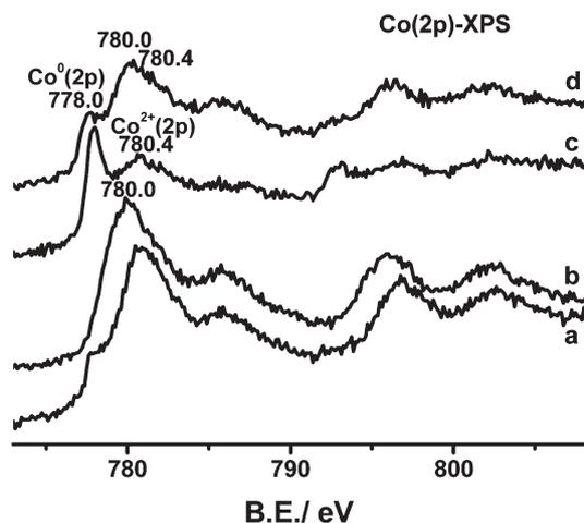
**Fig. 3** Co(2p)-XPS-spectra of the functioning catalysts: (a)  $\text{Co}_3\text{Cu}_1$  and (b)  $\text{Co}_3\text{Cu}_1$ -11%CNT, both fed with the  $\text{CO}_2$ -containing syngas:  $\text{H}_2/\text{CO}/\text{CO}_2/\text{N}_2 = 46/46/5/3$  (v/v); (c)  $\text{Co}_3\text{Cu}_1$  and (d)  $\text{Co}_3\text{Cu}_1$ -11%CNT, both fed with the  $\text{CO}_2$ -free syngas:  $\text{H}_2/\text{CO}/\text{N}_2 = 45/45/10$  (v/v).
