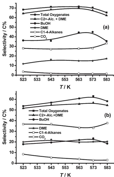
Fig. 1 Dependence of selectivity of products in the HAS upon temperature over: (a)  $\text{Co}_3\text{Cu}_1$ -11%CNT and (b)  $\text{Co}_3\text{Cu}_1$ ; at 5.0 MPa,  $\text{H}_2/\text{CO}/\text{CO}_2/\text{N}_2 = 46/46/5/3$  (v/v), GHSV = 10000 mL(STP)  $\text{h}^{-1}$   $\text{g}_{\text{cat}}^{-1}$ .
