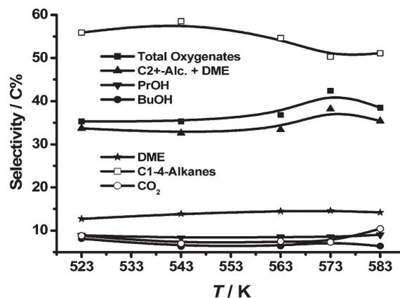
Fig. 2 Dependence of selectivity of products in the HAS upon temperature over  $\text{Co}_3\text{Cu}_1$ -11%CNT at 5.0 MPa,  $\text{H}_2/\text{CO}/\text{N}_2 = 45/45/10$  (v/v), GHSV = 10000 mL(STP)  $\text{h}^{-1}$   $\text{g}_{\text{cat}}^{-1}$ .
